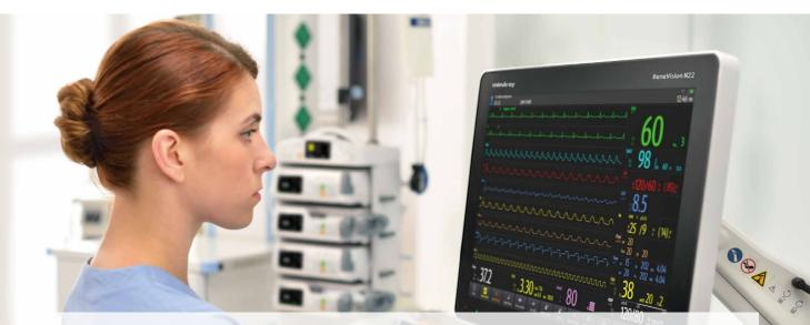
Mindray's Impedance Cardiography (ICG) module utilizes thoracic electrical bioimpedance (TEB) technology. The module continuously measures hemodynamic parameters such as cardiac output, system vascular resistance, heart contractility and thoracic fluid content non-invasively. ICG module significantly reduces the costs and eliminates or minimizes complications associated with invasive monitoring.
